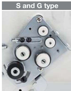
Thread tension controller for the LH-3528A-S and -G (standard type)
